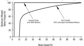
If external fan cooling is provided, open ventilated motors can also achieve an extended speed range at full rated torque. A box fan or blower with a minimum of 100 CFM is recommended. Mount the fan or blower so the motor is surrounded by the airflow. See Figure 4-2.
