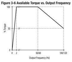
For 120Hz output with 60Hz motor, set J1 to the "60Hz" position and J2 to the "X2" position. For 100Hz output with 50Hz motor, set J1 to the "50Hz" position and J2 to the "X2" position. See Figure 3-7.
