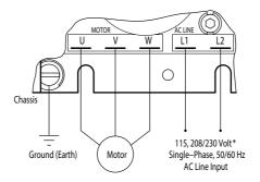
Connect the motor leads to terminals U, V and W. The terminals are located on the upper PC board. Motor cable length should not exceed 100 ft. (30 m) - load reactors may be required and must be ordered separately.
