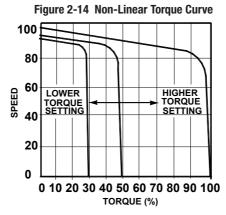
Because the BC200/BC201TM are regenerative controls, torque will be applied in both forward and reverse directions. The maximum torque can be set with the FWD CL and REV CL trimpots, and by using the FWD ACC and REV ACC trimpots, the rate of change of torque can be made more or less gradual. The maximum speed trimpot can be used to set the maximum motor speed under a no load condition.
