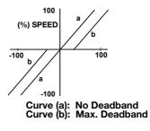
Note: If the deadband trimpot is set too low (CCW direction), the motor may oscillate between forward and reverse. Adjust deadband trimpot CW until the instability disappears. (Oscillation may also occur due to response setting.
