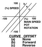
Figure 2-12 Deadband Trimpot Adjustment
