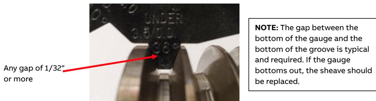
**Figure 2. Inspecting sidewall wear with a v-belt groove gauge**
