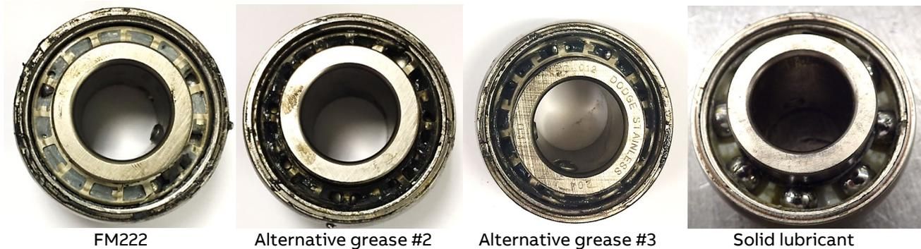
**Figure 2: Grease washdown comparison**
