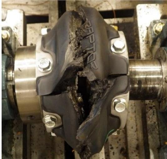
**Figure 3.** Excessive torque and misalignment
