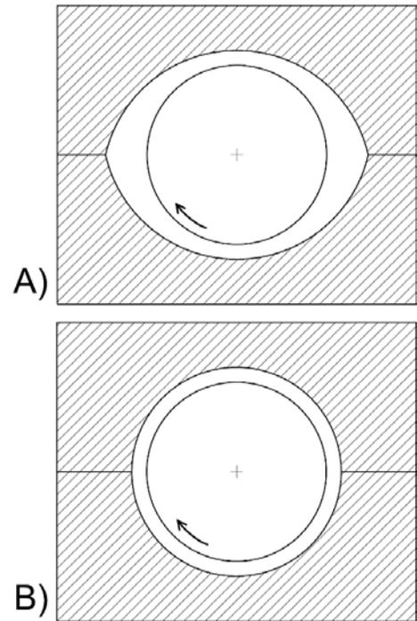
**Figure 6.** Common journal bearing profiles for fan applications are A) elliptical and B) cylindrical.
