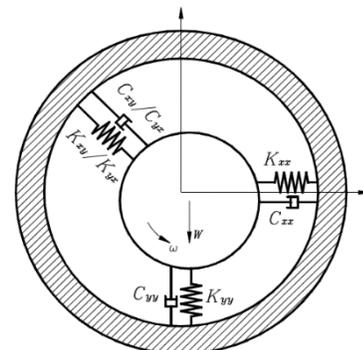
**Figure 3.** Spring-mass-damper model of a hydrodynamic bearing [2].
