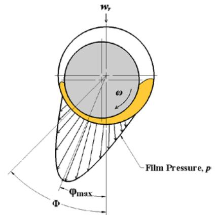
**Figure 1.** Pressure profile of a hydrodynamic bearing during normal operation.
