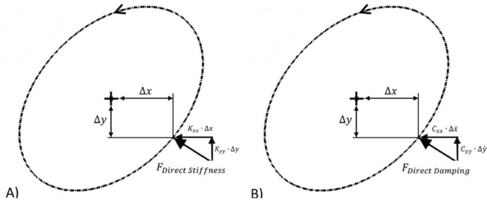
**Figure 5.** Forces caused by A) Direct Stiffness and B) Direct Damping and their relation to shaft orbit [2].
