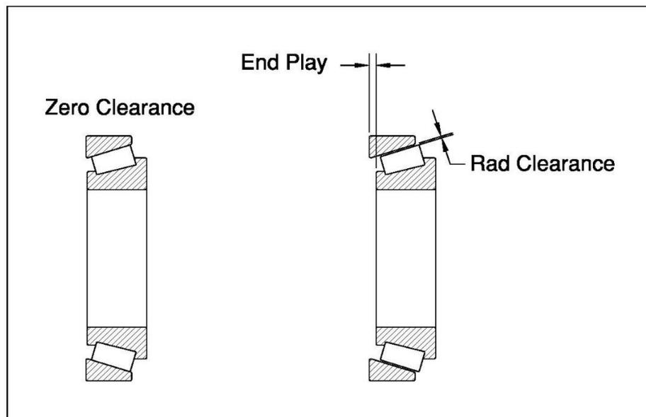
**Figure 2.** Tapered roller bearing with end play adjustment
