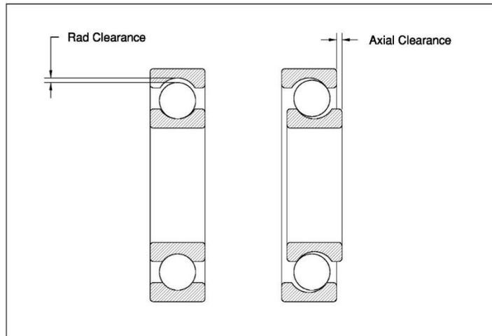
**Figure 1.** Internal radial and axial bearing clearance
