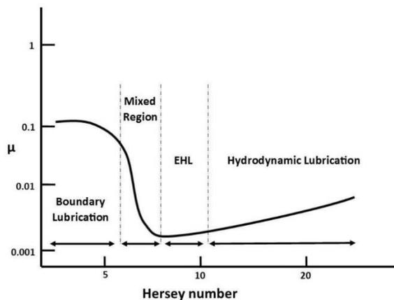
**Figure 1.** Stribeck curve comparing coefficient of friction with dimensionless Hersey number (Hamrock, Schmid, and Jacobson, 20014)
