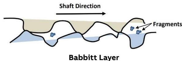
**Illustration 2.** The shaft surface asperities will break the liner surface asperities and leave broken Fragments that can advance bearing wear and failure
