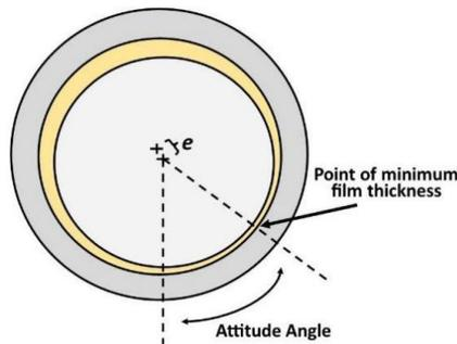
**Illustration 1.** Illustration showing the attitude angle and point of minimum film thickness
