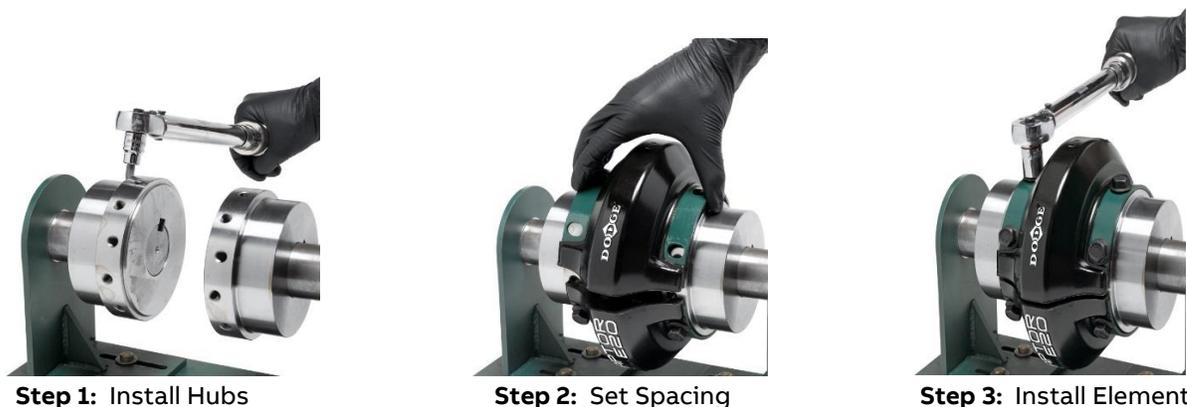
**Figure 1.** Installation is as easy as 1-2-3.
