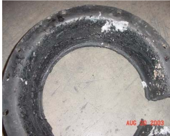
Figure 3: Degradation of Rubber Due to Excessive Vibration
