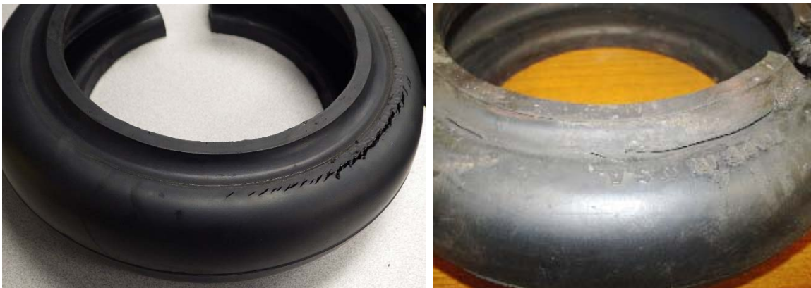
Figure 3: Tearing Commonly Associated with Excessive Misalignment
