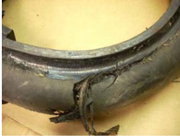
Figure 2: Tearing Commonly Associated with Cyclic Stress
