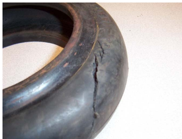
Figure 1: Tearing Commonly Associated with Excessive Torque
