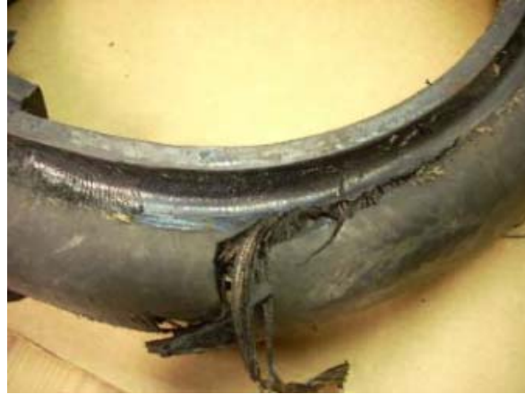
Figure 2: Tearing Commonly Associated with Cyclic Stress
