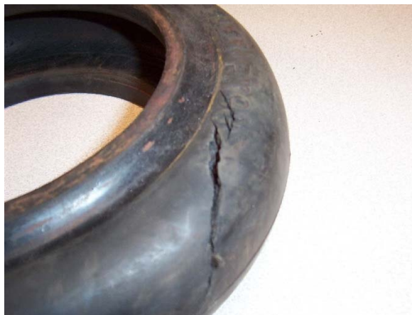
Figure 1: Tearing Commonly Associated with Excessive Torque
