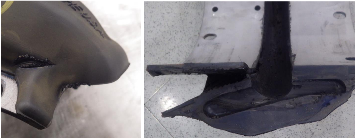
Figure 4: Typical tearing patterns at the element split as a result of excessive misalignment, torque, or vibration.
