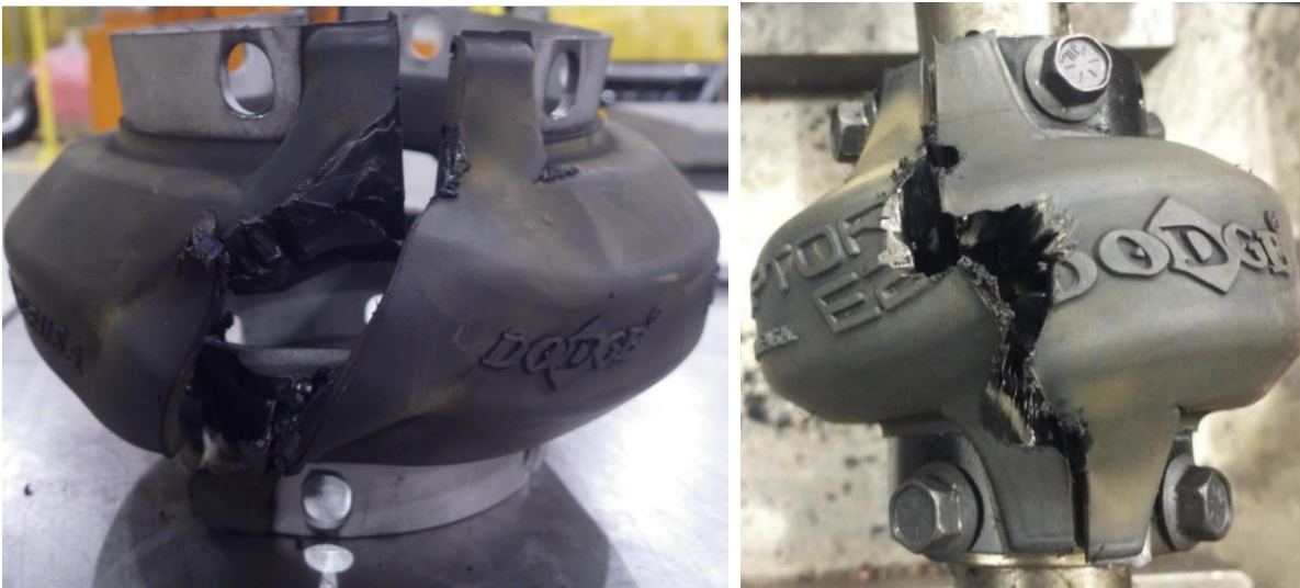
Figure 2: Typical tearing patterns at the element split as a result of excessive misalignment, torque, or vibration.
