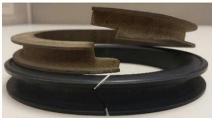
**Figure 4.** Cork (top) and HNBR Dust Seal (bottom)
