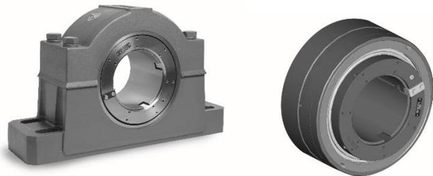
SAF style bearings are normally supplied with a labyrinth non- contact seal. Contaminants from the environment are kept out of the bearing by use of grease that fills the grooves between the seal and housing. The bearings must be 100% filled in order to have effective sealing. Dodge provides Triple Tech seals on their SAF style bearings that improve this standard seal by incorporating a V-ring seal that provides a contact sealing surface between the seal face and
