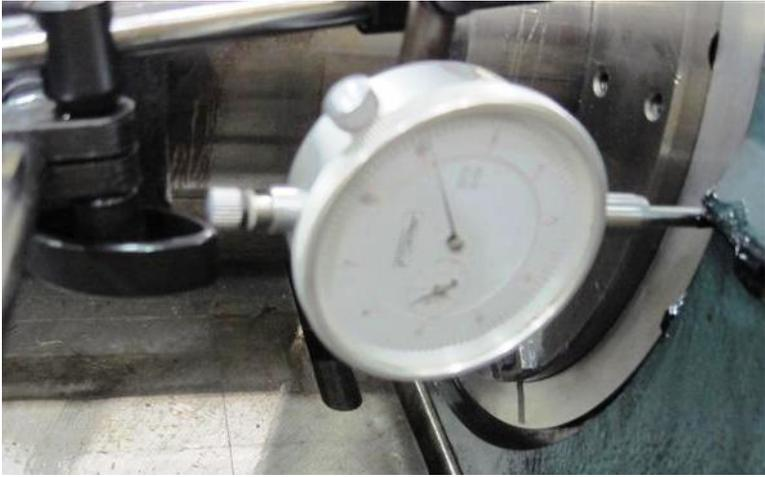
Figure 8: Dial Indicator at the 3 o'clock Position
