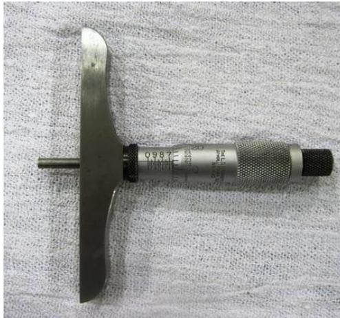
**Figure 3: Depth Micrometer**
