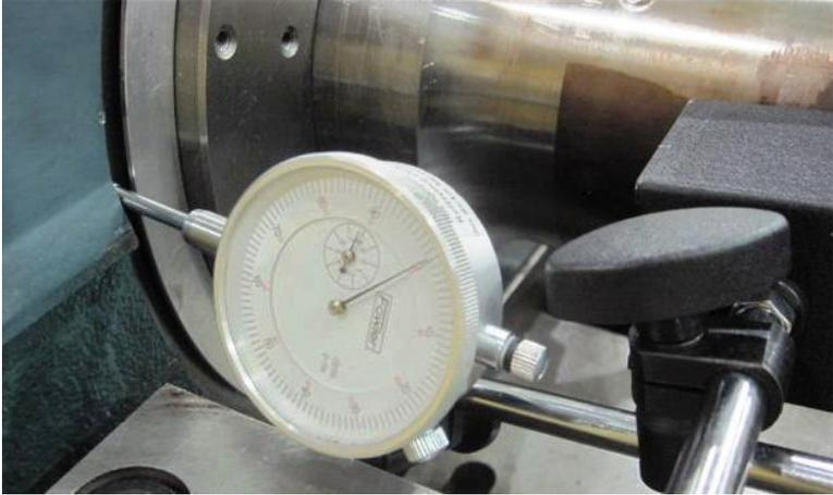
Figure 7: Dial Indicator at the 9 o'clock Position
