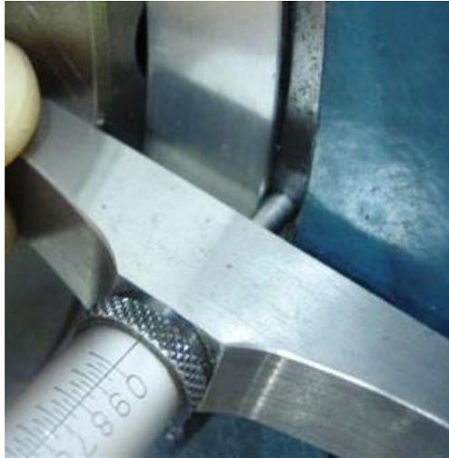
**Figure 5: Depth Micrometer at 3 o'clock position**
