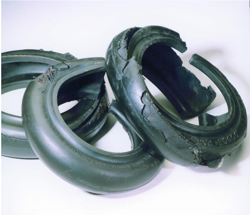
Figure #1: Torsional Overload Failures
