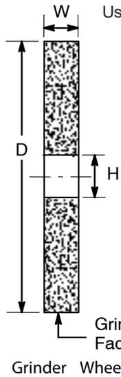
Use wheels rated at or over rated grinder RPM shown in the following table.
