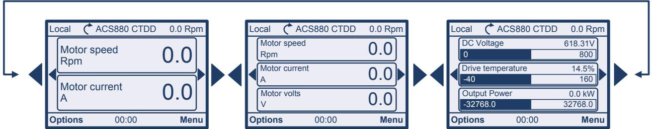
The Home view opens automatically when you power up the drive. The Home view is also displayed from the Options menu or the main Menu if no key is pressed for 10 minutes.
