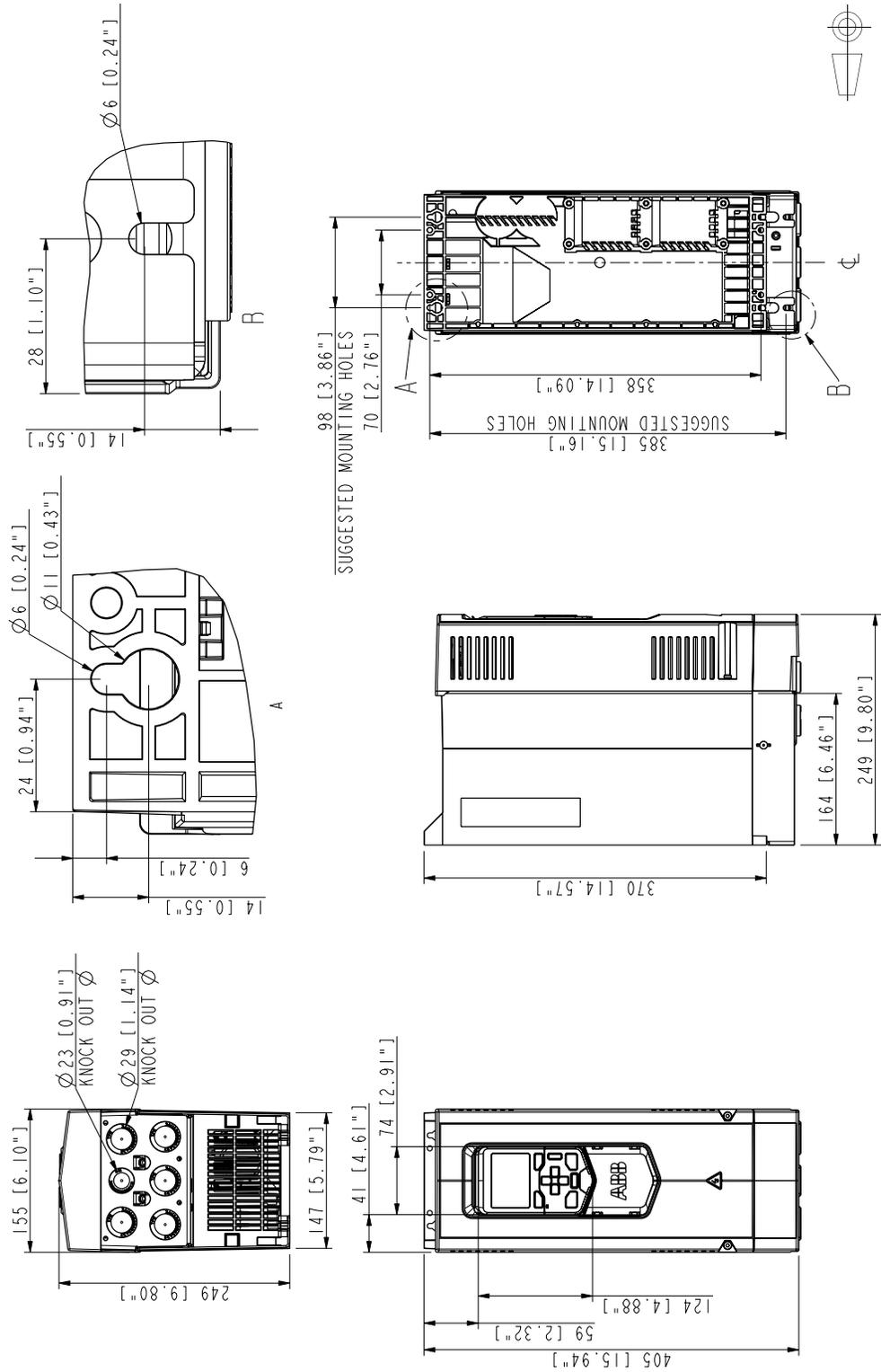
Figure B-3 Frame R3 (IP21, UL Type 1)
