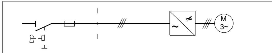
Size the fuses at the distribution board according to Table 5-2. The fuses will protect the input cable in short-circuit situations, restrict drive damage and prevent damage to adjoining equipment in case of a short-circuit inside the drive.
