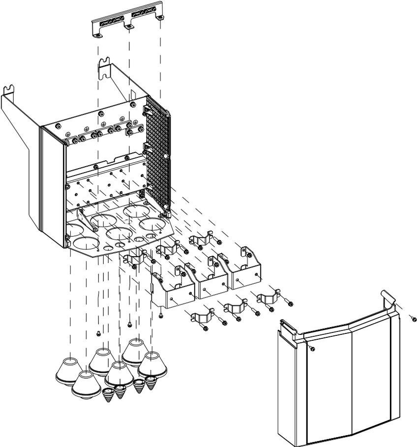
**D.6.4 Frame R9 Cable Entry Box (IP21, UL Type 1)**
