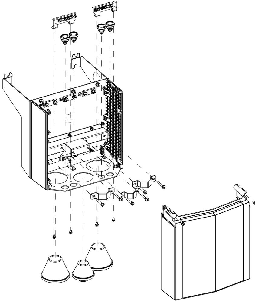
**D.6.3 Frame R8 Cable Entry Box (IP21, UL Type 1)**
