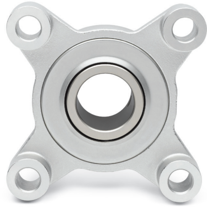
Figure 3 - Four bolt flange Stand-off bearing with Backside Seal installed. The even gap around the seal carrier and inner ring shall be maintained
