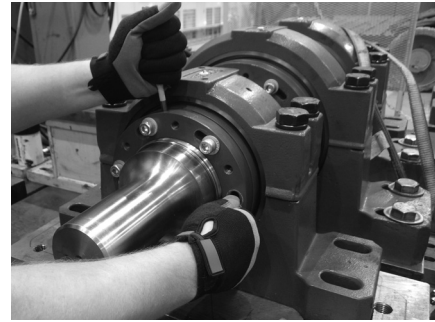
Figure 4 – Holding external nut and rotating internal nut using socket head cap screw
