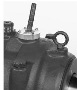
**Figure 5 - PLXC Circulating Oil Inlet**
