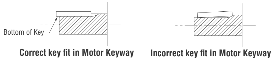
Figure 4 - Clamp Collar Motor Key Fit
