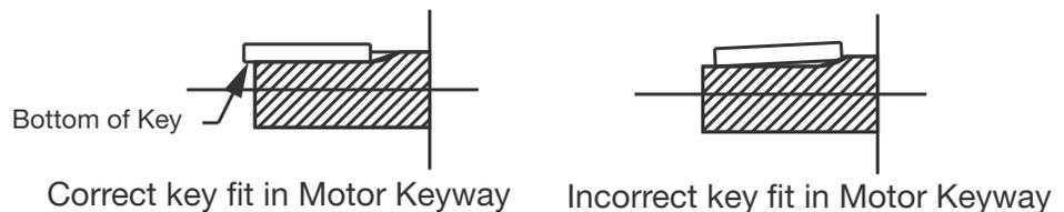
**Figure 5 - Clamp Collar Motor Key Fit**
