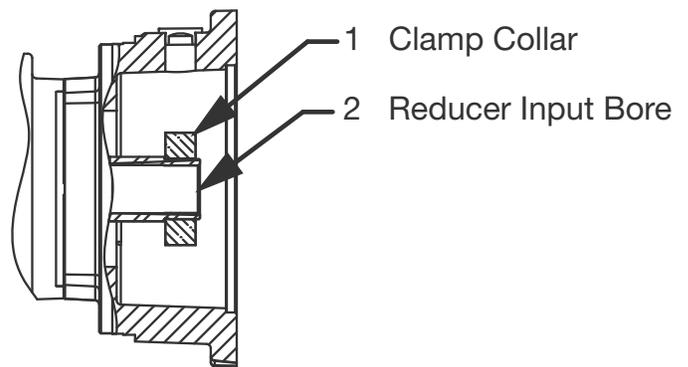
**Figure 4 - Clamp Collar Assembly**
