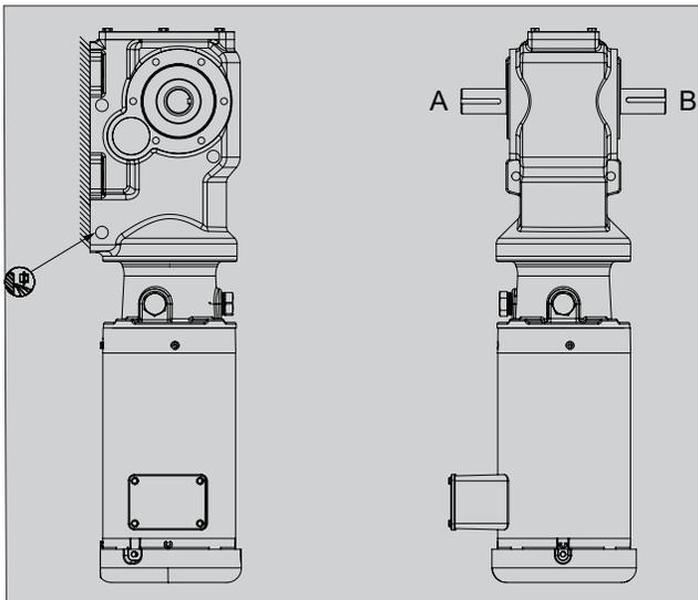
**NOTE:** Shaded A2 mounting is not a recommended mounting position due to the weight of oil on the highspeed input seal.
