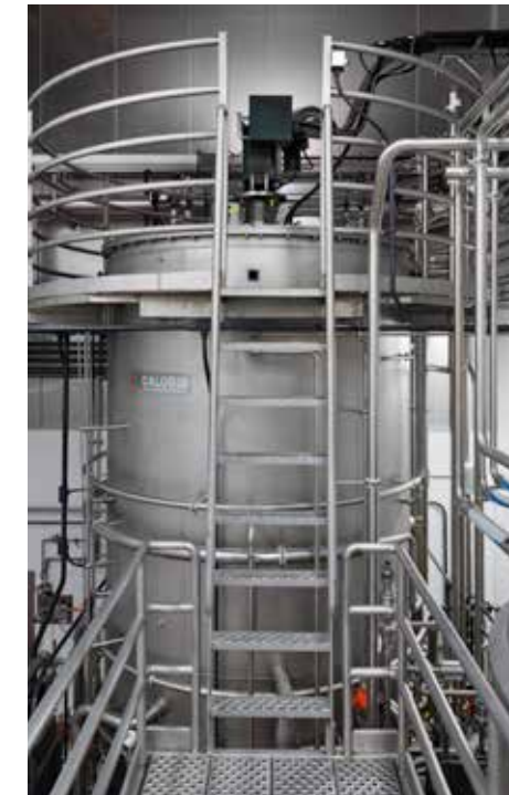
The Caloris Concentrix™ 200 evaporator utilizes proprietary turbofan technology in a highly efficient system that uses less energy and less water than traditional evaporation methods. Built in a concentric configuration, the Concentrix evaporator uses proprietary Caloris technology with a turbofan designed to efficiently discharge compressed heating vapors 360 degrees outward from the fan into the surrounding heat exchanger tube. This ultra-compact design takes half the space of other technologies to process the same volume, saving space and installation costs.
