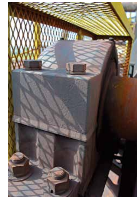
Baldor's Dodge Hydraulic ISAF pillow block bearing, with its patented, integral hydraulically assisted mount and dismount system, is quick and easy to install and remove. A built-in hydraulic piston is used on both the mount and dismount nut to facilitate tightening the bearing on the shaft during installation, and then aid in removal when it is time to dismount and replace the bearing. A harsh-duty, two-part sealing system protects the bearing from contamination and extends service life.
