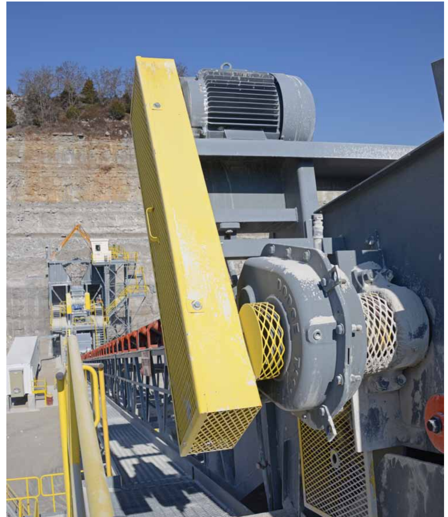
Considered the industry standard, Baldor's Dodge Torque-Arm II shaft-mounted speed reducers were selected for the project because of the product's proven performance and long-term reliability. The patented sealing system uses an HNBR oil seal protected by a metal excluder seal with rubbing lip, making this reducer a perfect fit for the harsh-duty industry.
