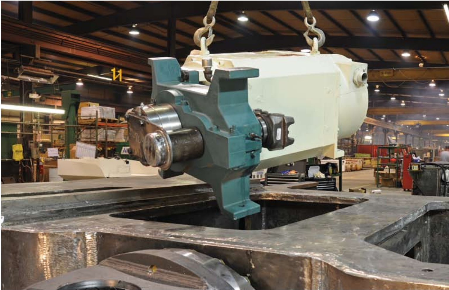
Fairchild International chose Baldor to help it move from DC to AC technology. Baldor engineers designed a gearbox (front of photo) with a new gear ratio to meet torque and speed requirements, while adding bearings built strong enough to handle the force of the application. The traction motor developed for the project is based on the Baldor•Reliance® RPM AC® product, with an optimized pole design, a robust sealing system to withstand underground environments and a feedback device for better speed control. The motor is also MSHA-approved explosion proof.
