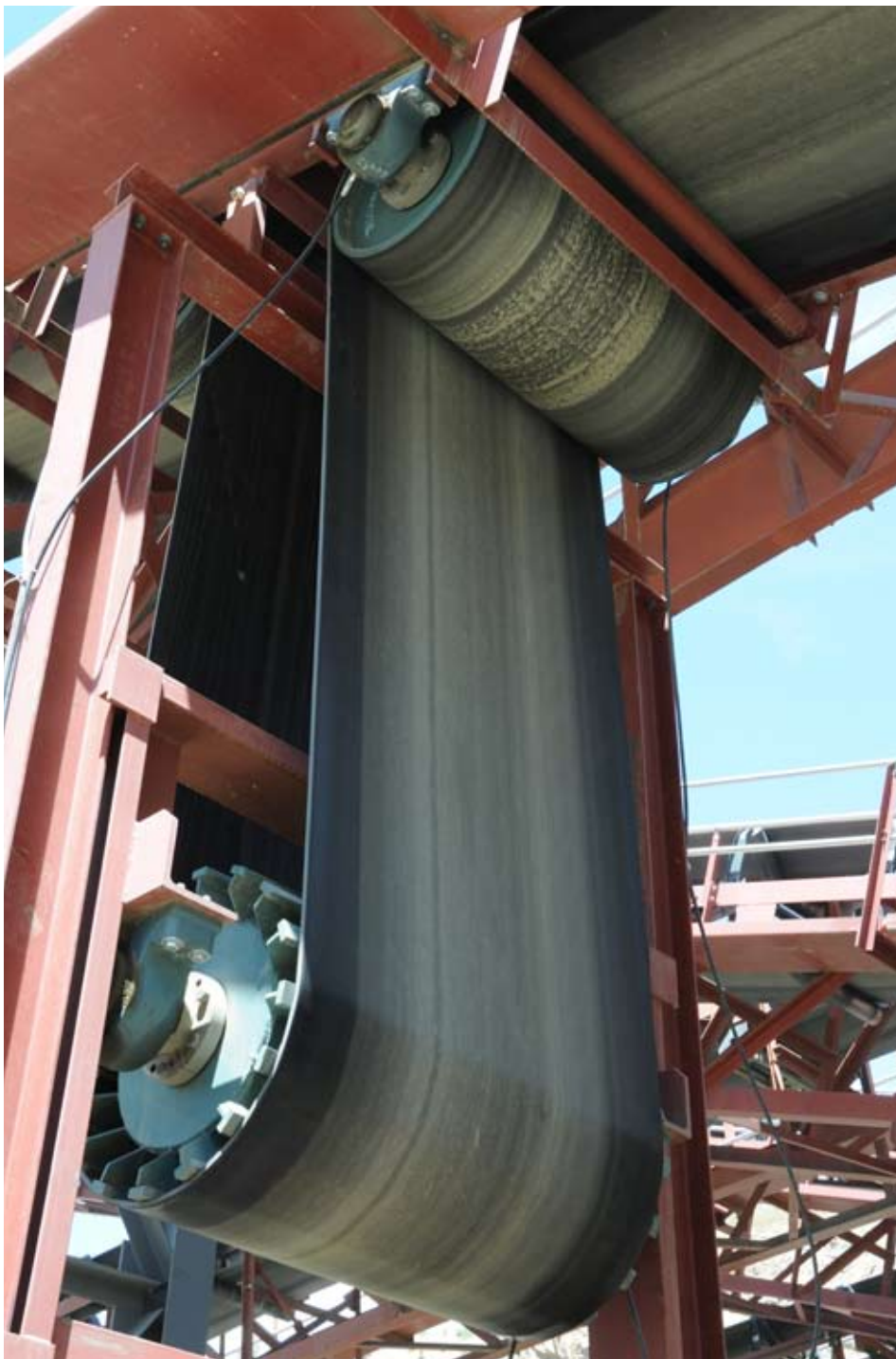
Both the Baldor•Dodge Mine Duty Extra wing pulleys (lower) and Mine Duty Extra drum pulleys (upper) use a thick, integral, one-piece hub design, eliminating the hub to end-disc weld, which is the most common failure point on a conveyor pulley. Albert Frei calls these pulleys rugged and tough.
