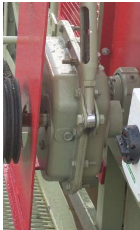
Dodge TORQUE-ARM II speed reducers' use of two-stage helical gearing makes the product 96% efficient, saving Corcoran Concrete energy.
