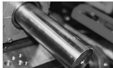
IMPERIAL bearing after 2500 hours
