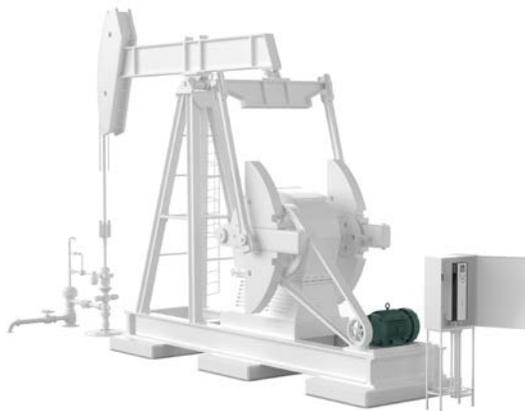
The most common method used for this purpose is the beam pump, the oldest type of artificial lift system. The beam pump is a version of a rod pump; as the beam moves up and down, the rod moves up and down in the well creating suction that lifts the oil to the surface.
