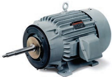
7.5-Hp, 3600-RPM TEFC close-coupled pump motor designed for low structure-borne vibration, with a threaded Monel® shaft per MIL-P-17840.
