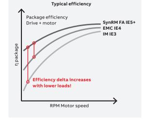
$\eta$  system =  $\eta$  drive  $\cdot \eta$  motor  $\cdot \eta$  coupling  $\cdot \eta$  fan  $\cdot \eta$  coil
