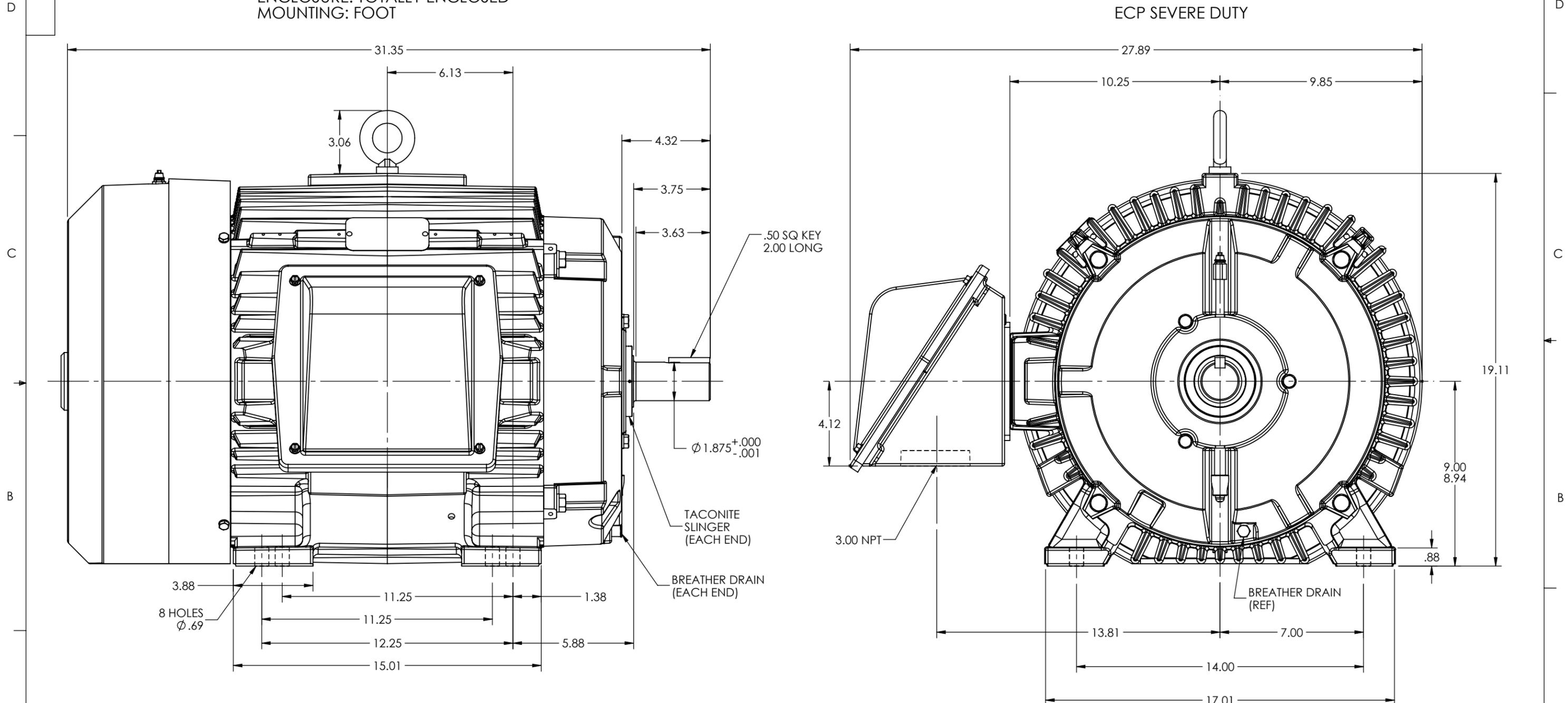
MAXIMUM PERMISSIBLE SHAFT RUNOUT WHEN MEASURED AT END OF STD. SHAFT EXTENSION IS .002 T.I.R. UP TO AND INCLUDING 1.625 DIA. AND .003 T.I.R. 1.625 DIA. TO 5 INCH DIA.
