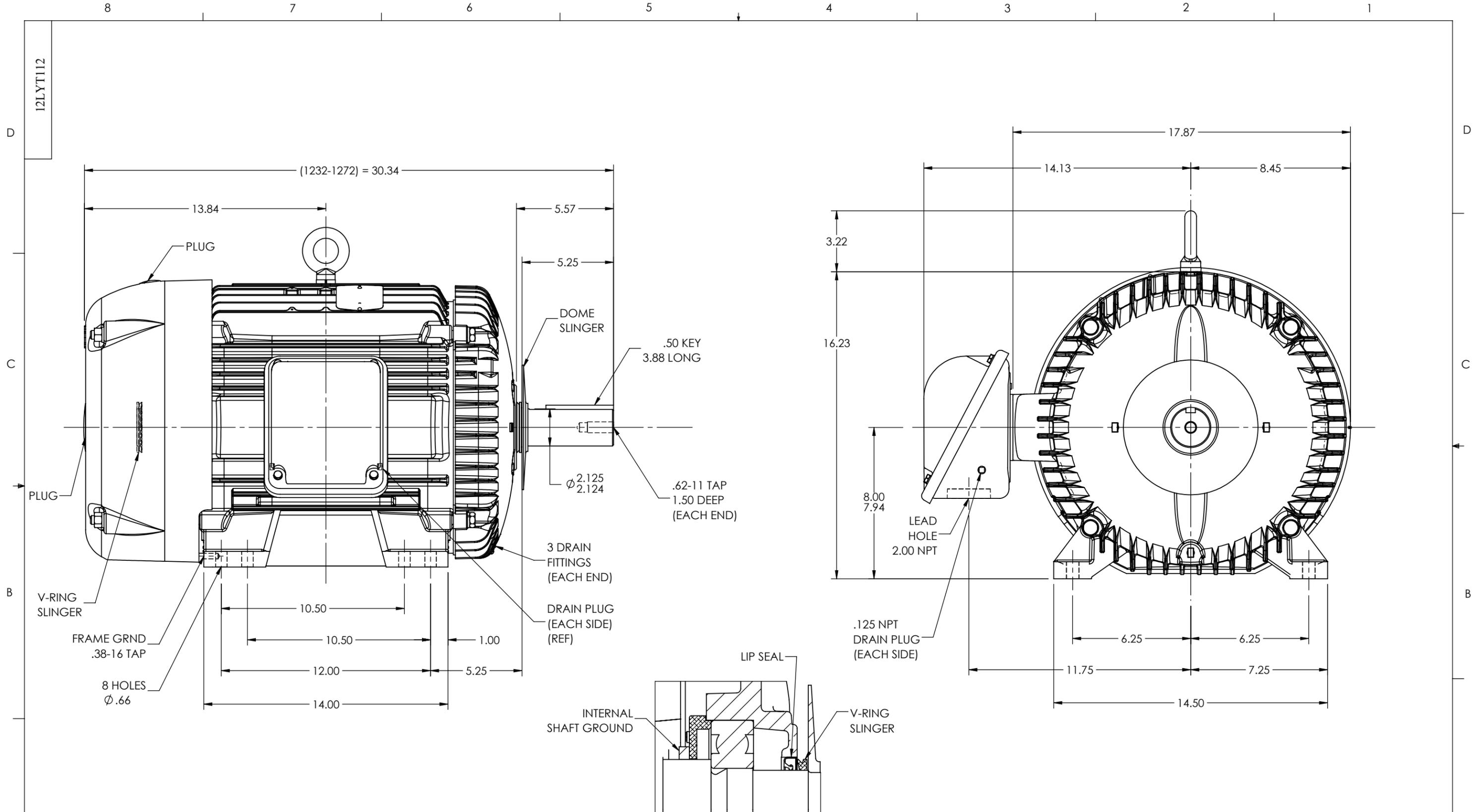
CUSTOMER ONLY NOTE: FOR VERTICAL SHAFT UP AND VERTICAL SHAFT DOWN LIFTING, REMOVE EYEBOLT FROM TOP OF MOTOR AND SCREW INTO END OF SHAFT.
