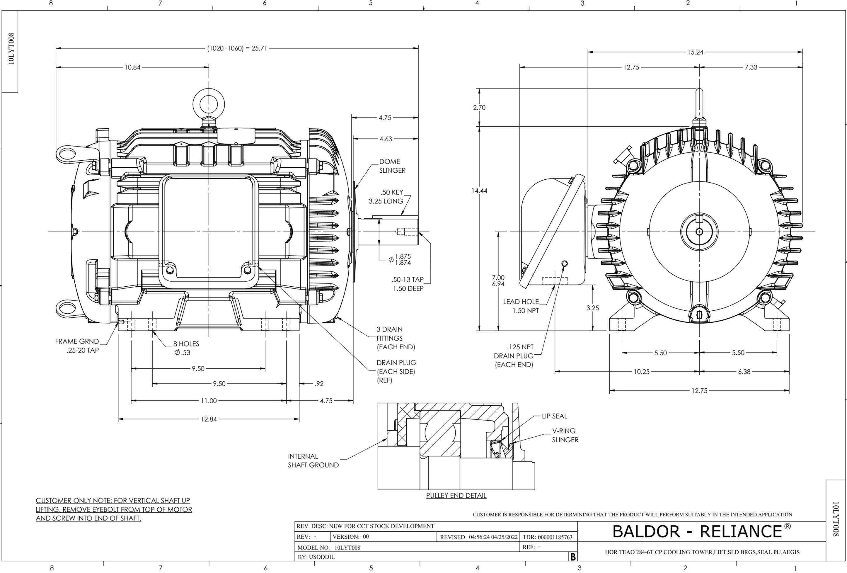
CUSTOMER ONLY NOTE: FOR VERTICAL SHAFT UP LIFTING, REMOVE EYEBOLT FROM TOP OF MOTOR AND SCREW INTO END OF SHAFT.
