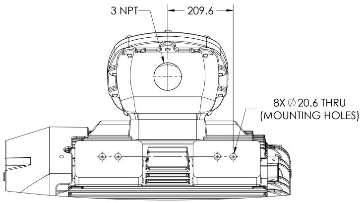
DIMENSIONS ARE IN MILLIMETERS. WEIGHT (KGS): 975, MOTOR WEIGHTS MAY VARY BY 15% DEPENDING ON RATING.
