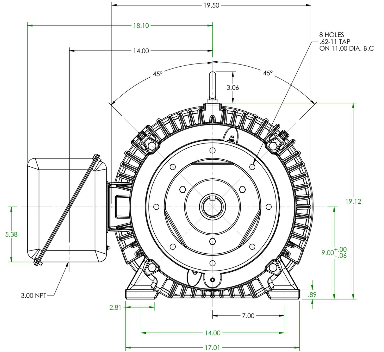
MAXIMUM PERMISSIBLE SHAFT RUNOUT WHEN MEASURED AT END OF STD. SHAFT EXTENSION IS .002 T.I.R. UP TO AND INCLUDING 1.625 DIA AND .003 T.I.R. 1.625 DIA. TO 5 INCH DIA.
