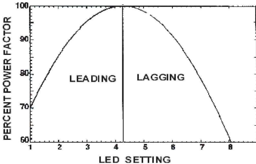
**FIGURE 7B - POWER FACTOR ADJUSTMENT**
