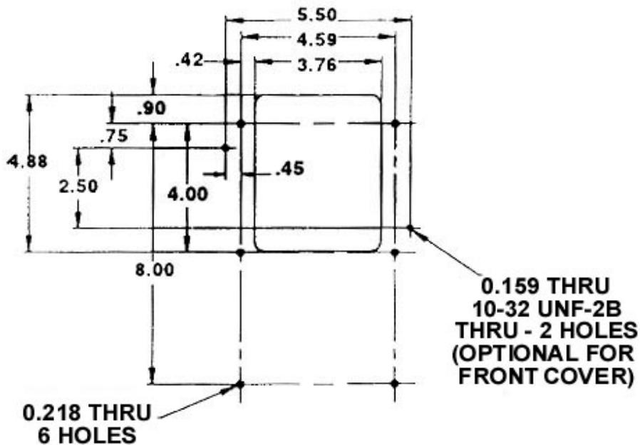
**FIGURE 4 - REGULATOR MOUNTING DIMENSIONS**
