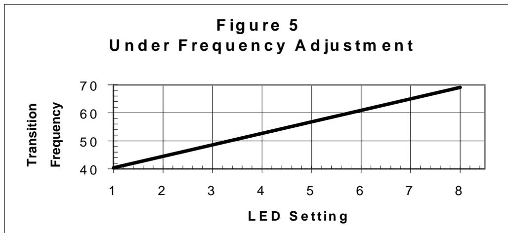
To set the transition level to a known frequency, either of two (2) methods of adjustment may be used.
