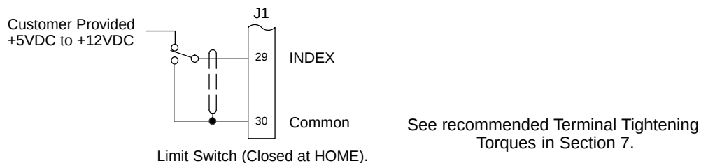
Figure 3-26 Typical Home or Orient Switch Connections
