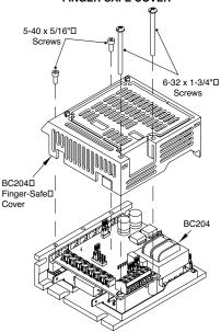
Use the two (2) 6-32 X 1-3/4" screws previously removed to secure the BC215 to the BC204. Do not over tighten these screws or damage may result to the BC215 and BC204. See figure 3 on page 7.
