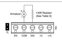
TABLE 3 – RESISTOR FOR SIGNAL FOLLOWING FROM ARMATURE VOLTAGE
