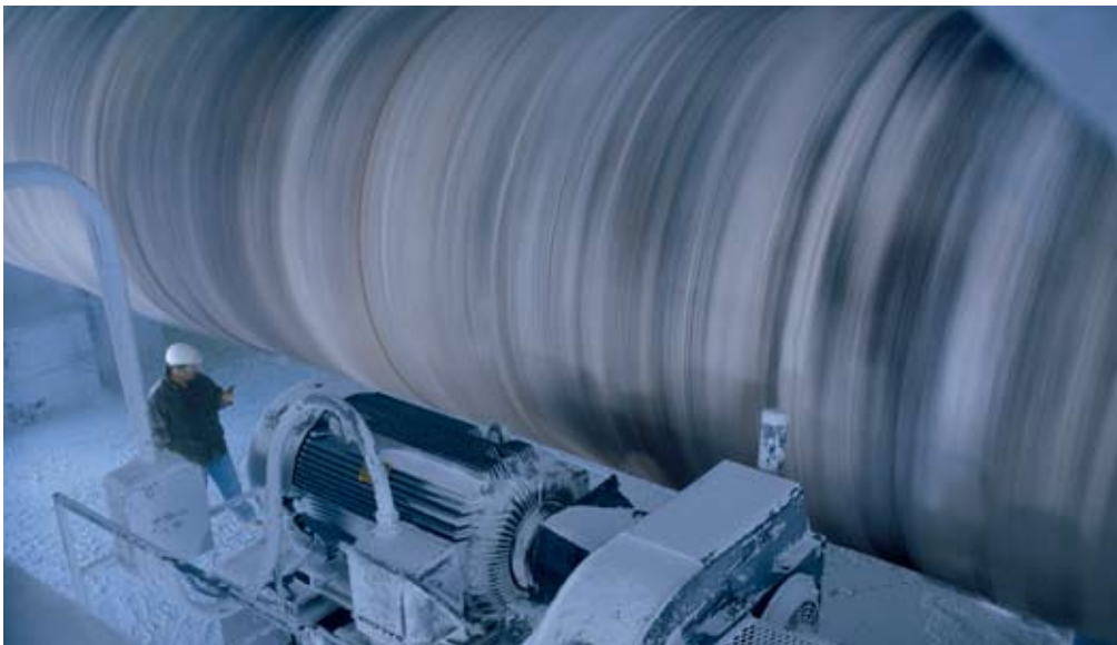
A Baldor 500 Hp, totally enclosed fan cooled motor drives this giant rock tumbler at a marble plant.
