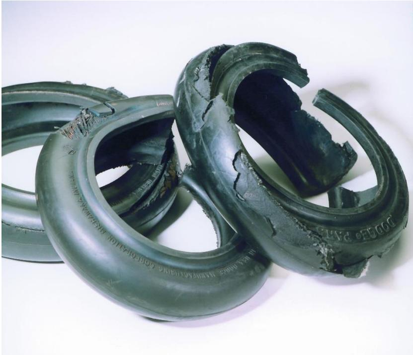
Figure #1: Torsional Overload Failures
