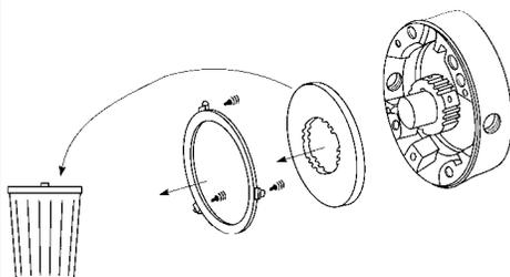
**4** Reposition support plate on endplate and tighten mounting screws to 55 lb-in.
