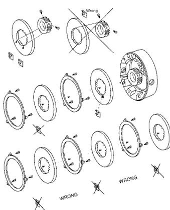
**Note:** Stabilizer clips should never be located over the set screws of the hub.
