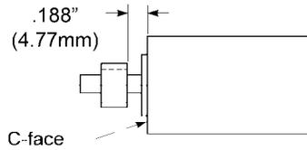
**3** Tighten set screws to motor shaft.
