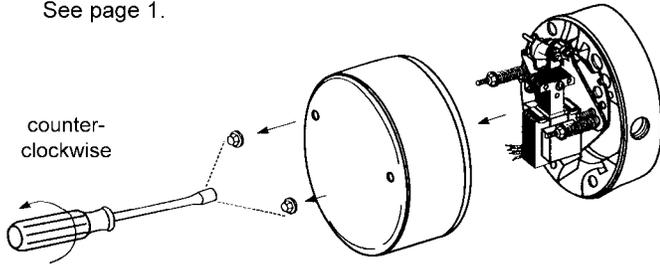
**5** Slide endplate over hub noting position of stabilizer clips, if used. (Refer to Friction Disc Replacement, view 3 and 3A.) Tighten mounting screws.
