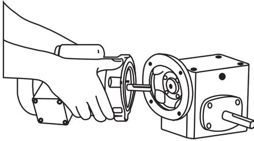
**STEP 2.** Tighten the supplied 4 bolts with lockwashers evenly for a solid fit between motor and "C" flange.
