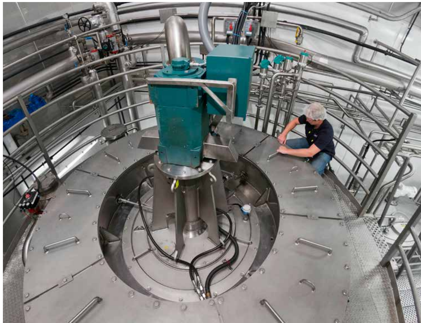
A drip-proof, forced-ventilated Baldor•Reliance RPM AC motor with a permanent magnet rotor was selected to power the proprietary turbofan technology on the Caloris Concentrix™ 200 evaporator. RPM AC motors feature a unique laminated steel, square-frame construction and a premium insulation system to provide ultimate torque performance in a compact package. RPM AC motors can be designed for specific horsepowers and speeds to provide the ultimate in system matched performance.
