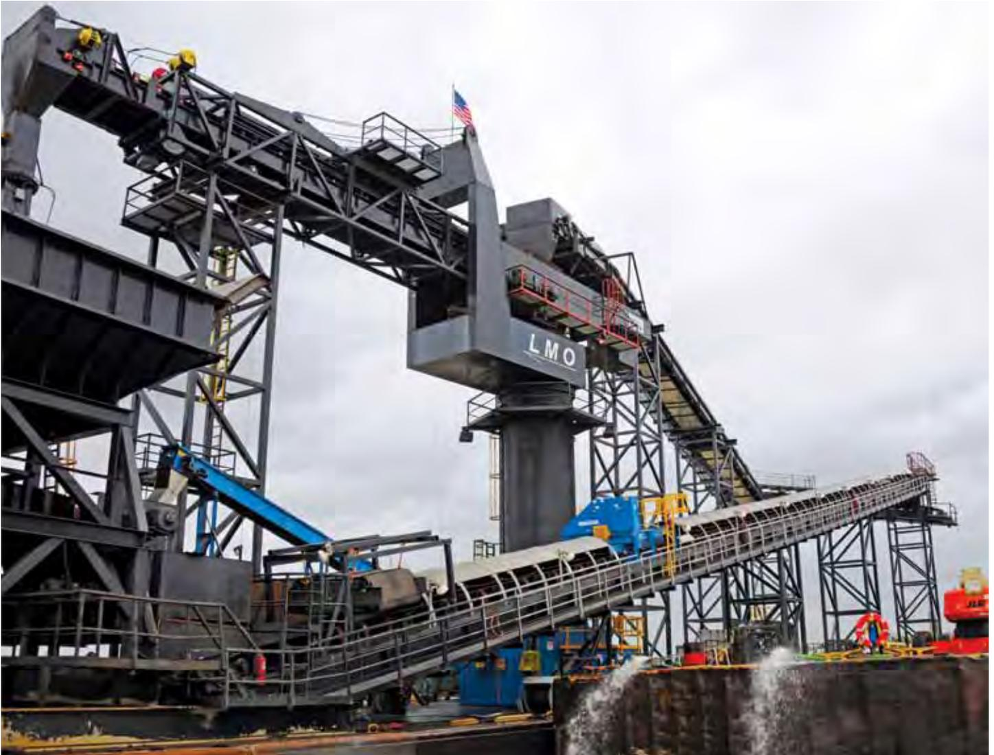
The Louisiana Mid-Stream One (LMO) is a unique barge-mounted conveying system with quality control features not found in other midstream loading operations, including a magnet, mechanical sampling system, belt scale and water drainage. The LMO can simultaneously feed and combine product from multiple barges to meet quality specifications, enhancing the quality of export coal.
