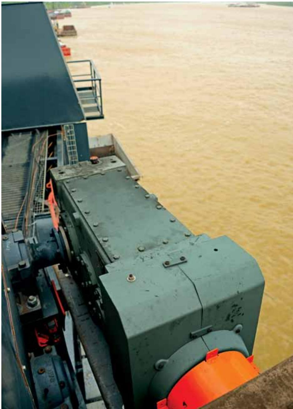
Not only did the customer get the MagnaGear reducers in three days, but Jim McLain, with Allied Bearing & Supply, says the customer got a product much better suited for this application. He says the MagnaGear reducers provide twice the output torque than the boxes they replaced, plus the right-angle configuration of the reducer is a perfect fit for this conveyor design.
