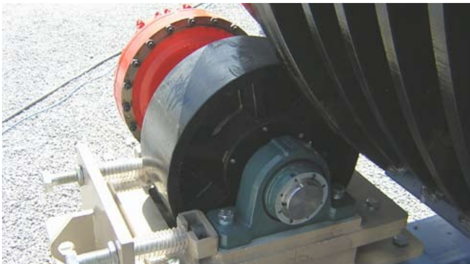
Stalex Construction Equipment, manufacturer of the renowned Hercules range of trommels, has standardized on Baldor•Dodge Imperial ISN bearings for all the main rotational load-bearing parts on its new HT182M road-going trommel.
