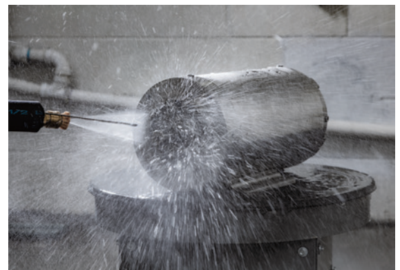
TENV SSE motor being tested for IP69K
