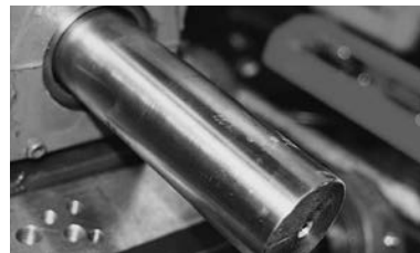
IMPERIAL bearing after 2500 hours
