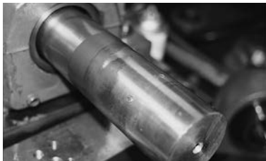
Setscrew Bearing after 500 hours
