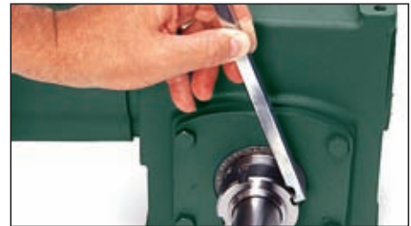
Complete locking procedure with hammer and drift
