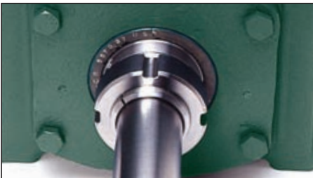
Slide bushing and reducer onto shaft.
